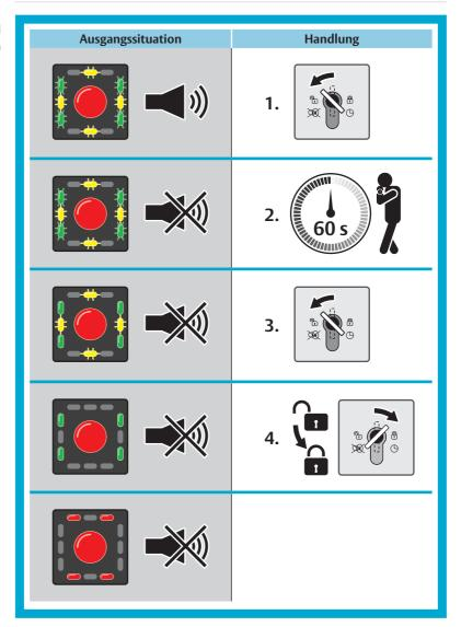
A function test is performed automatically depending on the cause of fault. If the fault has been corrected and functionality has been re-established, the escape route securing system will be locked automatically in order to test the function of the system components.
