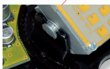
Radar module that is horizontally and vertically tiltable
